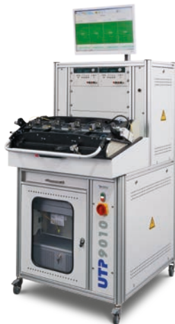
UTP 9010 RF EOL FOR TESTING AUTOMOTIVE INFOTAINMENT AND ECALL MODULES
