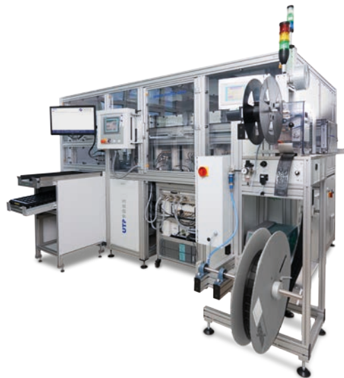
UTP 9085 IN-LINE-STATION FOR MULTI-DUT FLASHING, RF CALIBRATION & VERIFICATION
