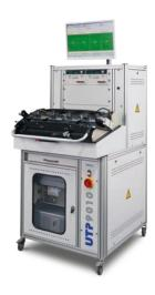
UTP 9010 RF EOL FOR TESTING AUTOMOTIVE INFOTAINMENT AND ECALL MODULES
