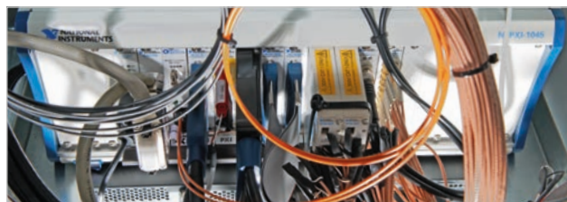
Internal wiring on the PXI core system
